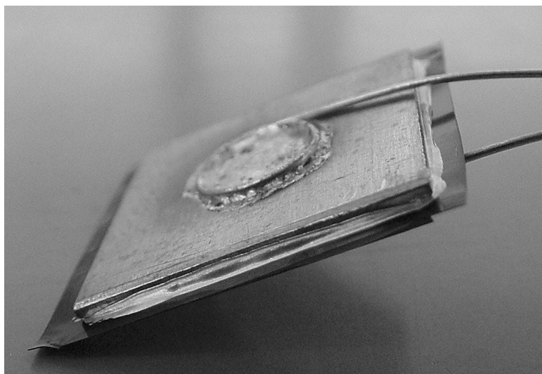
Figure 5. Glue sample used for the determination of the normal conductivity ( 20 \times 20 mm). Material buildup: copper electrode, glue, film, glue, and copper electrode.
